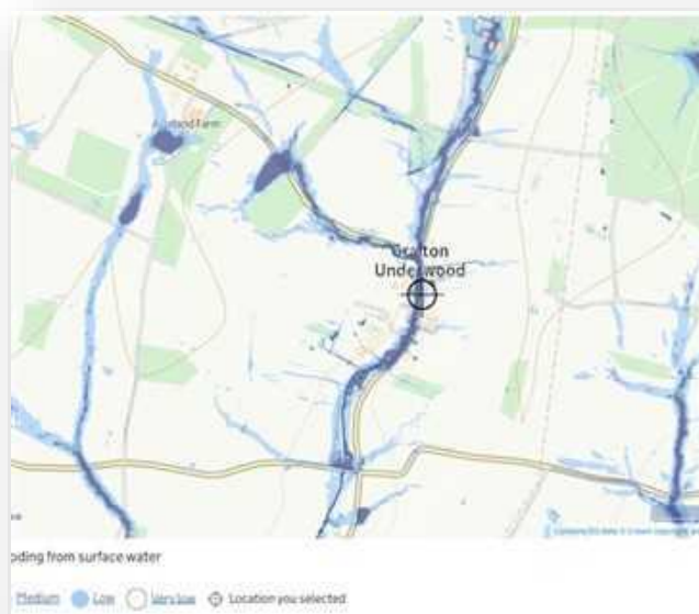
Figure 11: Extent of Water Flooding in Grafton Underwood
